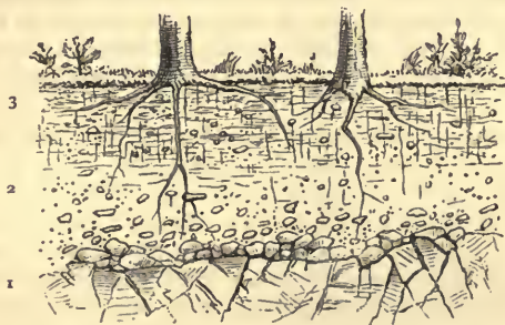
FIG. 25.—Section to show the formation of (3) soil and (2) subsoil from rotting away of (1) rock underneath.
